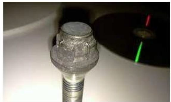
Examples of Damaged Screws
