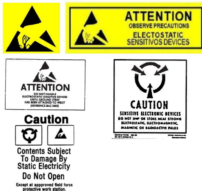
Examples of Label Identifying Electrostatic Discharge Sensitive devices Figure 2001/GRAPHIC-25-11-96-991-201-A01
