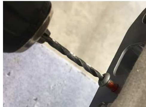
Damaged Screw Removal
