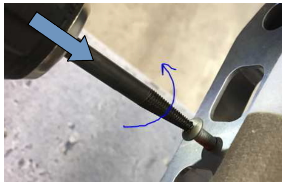
Damaged Screw Removal
