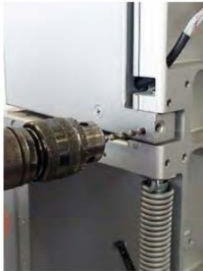
PROCEDURE FOR THE OLD SPRING P/N 153500-03 INSTALLATION Figure 7012/GRAPHIC-25-11-79-991-712-A01
