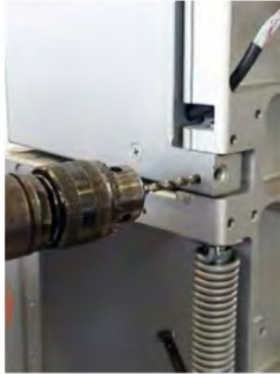
PROCEDURE FOR THE OLD SPRING P/N 153500-03 INSTALLATION Figure 7012/GRAPHIC-25-11-49-991-712-A01
